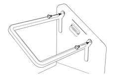
Use the provided screws to secure the arm.
