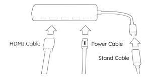
Plug the cables into the Hub as shown.
